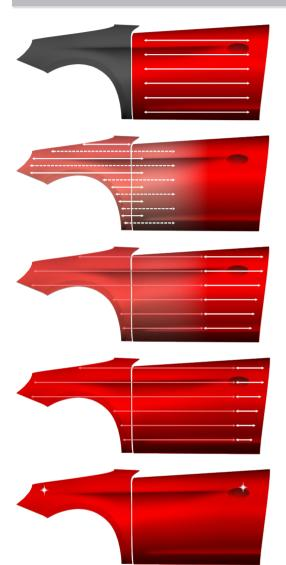
Adjacent panel: sand panel with suitable abrasive e.g. Trizact – P1000 New part / repair: sand surfacer (minimum P500)
